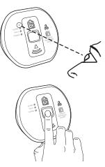
To test the RadioLINK<sup>+</sup> system, press and hold the test button on one of the Alarms. The blue LED from the Ei200MRF will illuminate for approximately 3.5 seconds. Continue to hold the test button until all the Alarms in the system are sounding. This will take a few seconds depending on the number of Alarms and their locations in the system, e.g. a system with 12 Alarms may take up to 45 seconds for all to sound. Release the test button when the test is completed.
