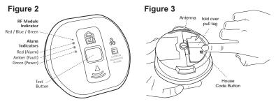
You can exit this mode by pressing the House Code button on one of the RF Alarms. Keep the button pressed until the blue light comes on solid and then release. Now re-affix the Alarm to its mounting plate.
