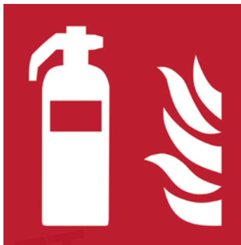
Fire extinguishers in accordance with ISO 7010
