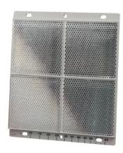
The 6500R and 6500RS are conventional reflector type linear optical beam smoke detectors designed to operate as a component of an non-ddressable fire alarm system. It operates primarily on the principle of light obscuration utilising infra-red light. Optical beam smoke detectors are particularly appropriate for protecting buildings with large open spaces such as warehouses, atriums etc.
