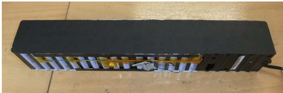
Figure 1. Battery pack in 13s6p connection
