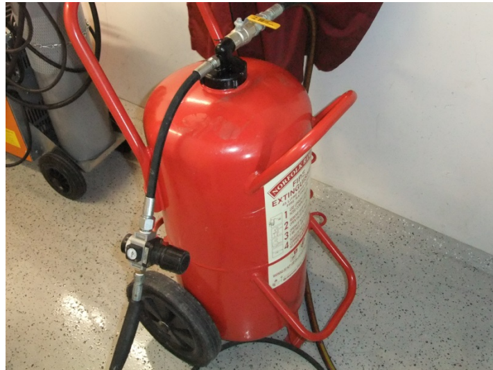
Figure 6: Pressurised reservoir for the fire extinguishing agent (AVD)
