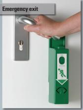
While using the door handle the GfS Exit Control 179 drops down vertically. It is possible to use the emergency exit with one single grasp. A permanent alarm signal is triggered. It is switched off with the key.
