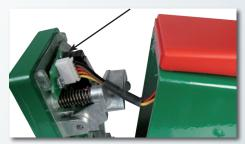
Open the housing slowly and pull out the cable of the radio transmitter.
