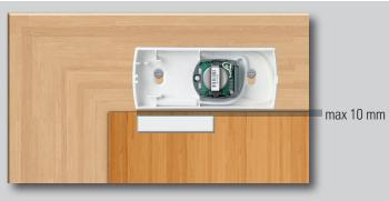
3. Mount the counterpart with the raw magnet parallel to the reed contact. **The distance should not be more than 10 mm!**
